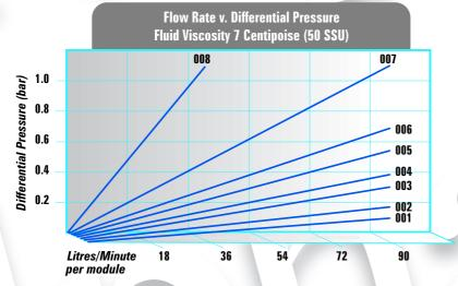
Still exhibiting a high flowrate per unit area, Alphacel can be used for clarifying any type of spirit, solvent or light oil fraction, particularly useful in the distilling industry and petrochemicals.
