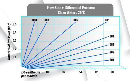
Alphacel exhibits a very high flowrate per cartridge, greater than the same area of media mounted in a filter press. This is due to the open nature of the media support within the cartridge cell, and the cell's ability to stand a high pressure differential without rupture.
