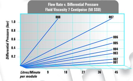
Still exhibiting a high flowrate per unit area Alphacel can be used for clarifying any type of spirit, solvent or light oil fraction, particularly useful in the distilling industry and petrochemicals.
