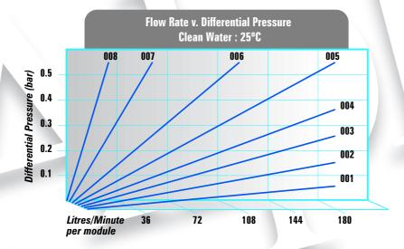
Alphacel exhibits a very high flowrate per cartridge, greater than the same area of media mounted in a filter press. This is due to the open nature of the media support within the cartridge cell, and the cell's ability to stand a high pressure differential without rupture.
